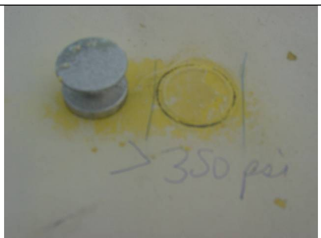
FIGURE 10. Adhesion Pull Test on Original Coating.
