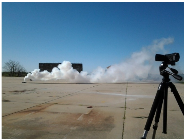
Figure 3. Field test of a typical end-burning BC prototype grenade. Grenade PH2-3-2 at 25 s (total burning time 61 s).
