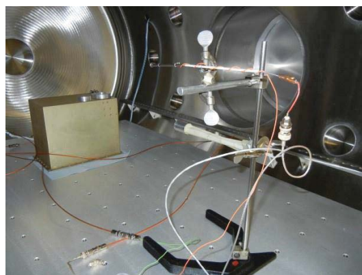
Figure 67. Langmuir Probe in Plasma Chamber
