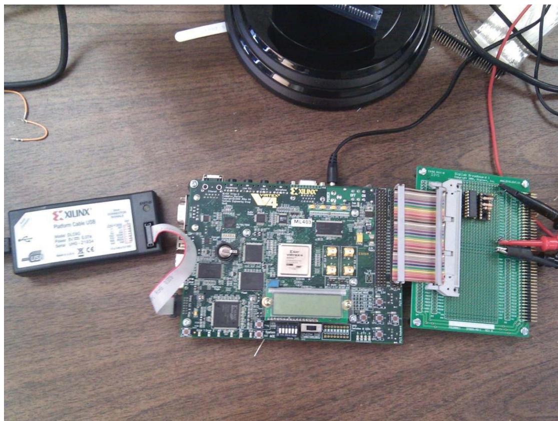
Figure 90. FPGA board connections where The FPGA board output is connected to the antenna input
