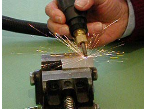
Figure 5. Application of ESD Coating to Test Coupon at OC-ALC.
