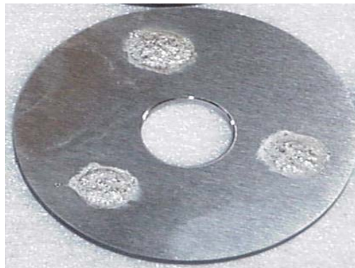
Figure 9. Pin-on-Disk Wear Test Specimen After Defects Repaired Using ESD but Prior to Surface Finishing.
