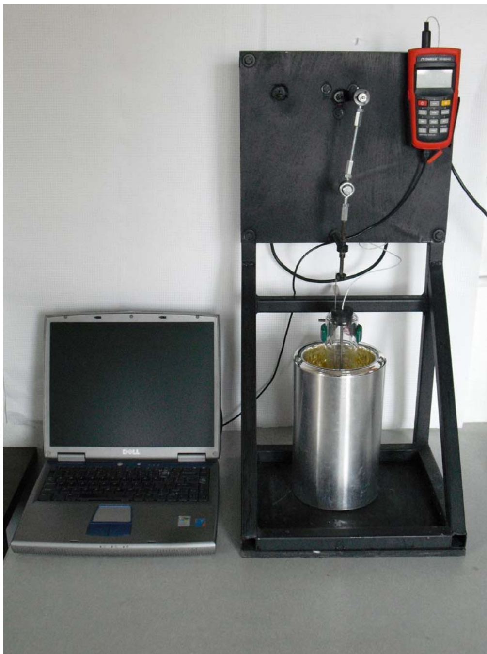
Figure A1. Photograph of freezing point apparatus built in accordance with ASTM D 1177.
