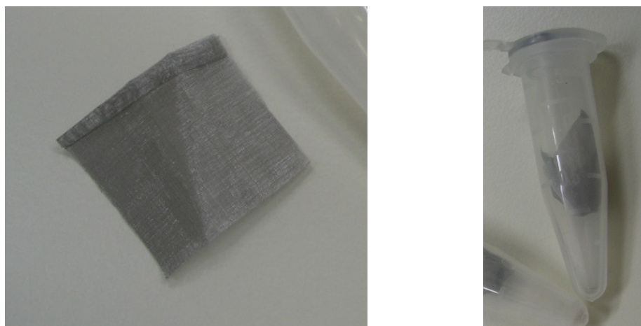
Figure 21. (left) Stainless steel mesh (2 cm \times 2 cm), as used; (right) tube containing the screen rolled into a cone, inserted in the tube.
