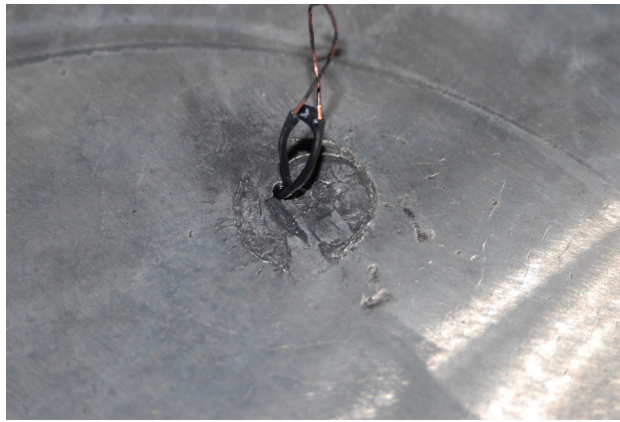
Figure 5. Denting above the explosive charge at the initiation wire port
