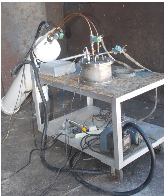
Figure 13. Dual-chamber system connecting vacuum chamber (81 liters) to detonation chamber (8.5 liters) to atmosphere via remote-controlled solenoid valves
