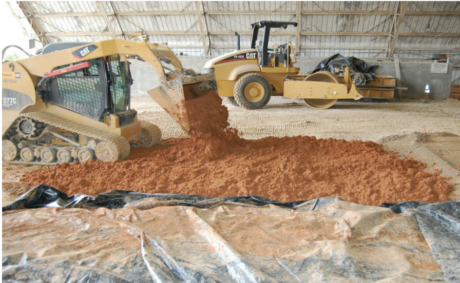
Figure 11. Placing a soil in the test section using a skid steer.
