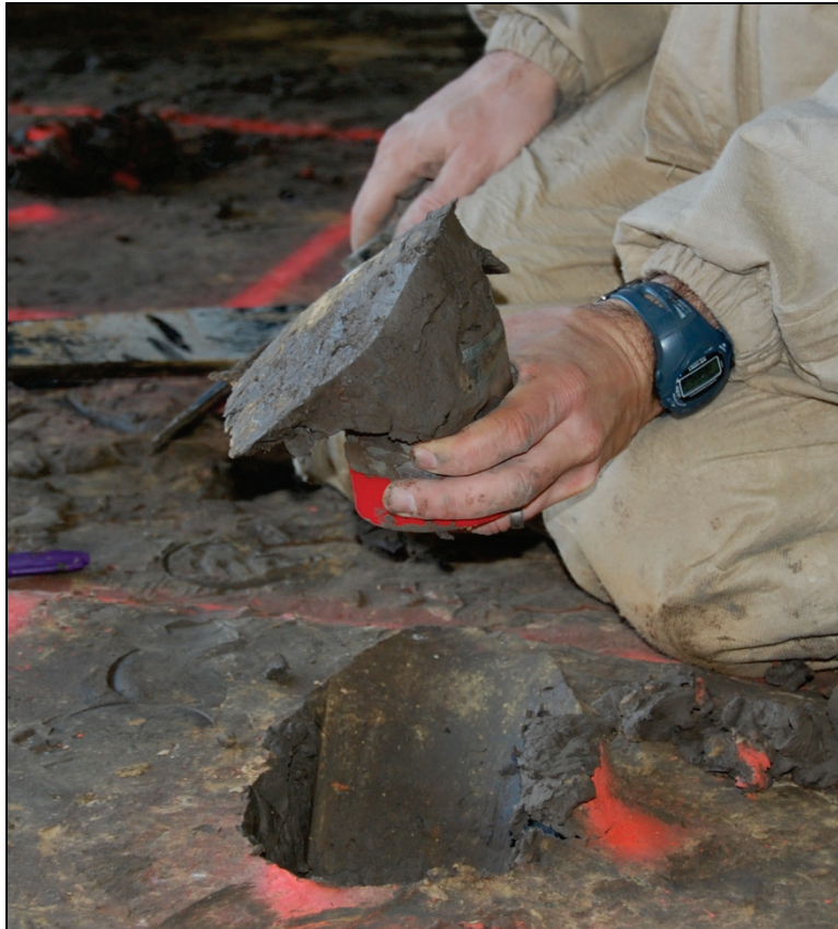
Figure 17. Conducting drive cylinder test in the buckshot clay.
