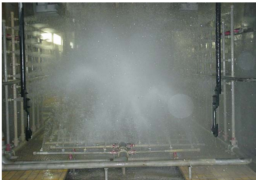
Figure 23. Typical spray application of zirconium pretreatments using risers.
