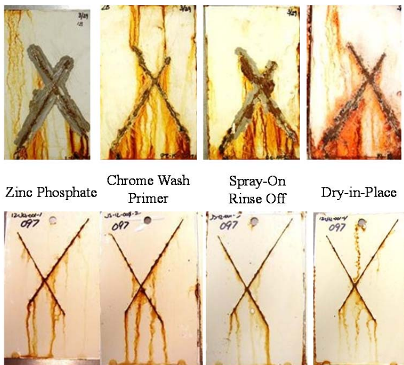
Figure 32. (top) Benchmark ASTM B117 Salt Spray Corrosion Testing (1000 hours) of the zirconium Spray-On/Rinse-Off and Dried-In-Place field-applied Treatments on CRS under MLN1981T MIL-DTL-53022B solvent-borne epoxy primer. (bottom) Benchmark GMW14872 Cyclic corrosion Testing (40 cycles) of the zirconium Spray-On/Rinse-Off and Dried-In-Place field-applied Treatments on CRS under MLN1981T MIL-DTL-53022B solvent-borne epoxy primer.
