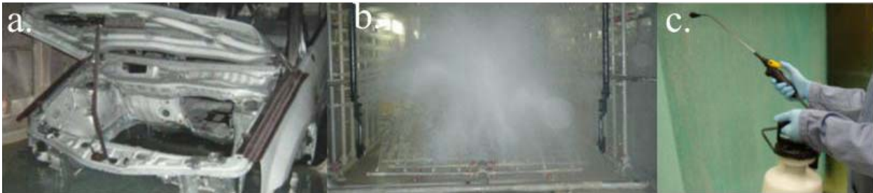
Figure 1. (a) Immersion application of zirconium pretreatments. (b) spray application of zirconium pretreatments. (c) Dried-In-Place application of zirconium pretreatments.
