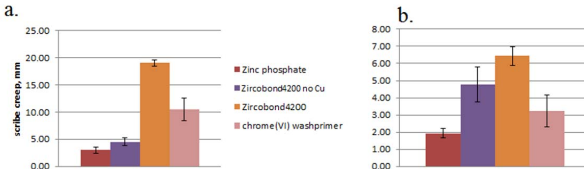
Figure 8. Four hundred hours neutral salt spray (a) and 20 cycles GMW14872 (b) of various pretreatments with a solvent borne (SB) primer system.
