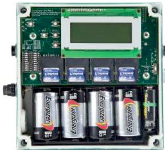
Figure 39. Wildlife Acoustics Song Meter SM2 recorder. The SM2 can be programmed to record on simple time-of-day schedules or more complex monitoring protocols such as recording relative to local sunrise, sunset and twilight. This unit accepts an external microphone for flexible deployment.
