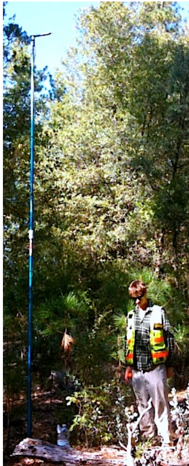
Figure 45. Bat detector remote microphones enable placement up and away from ground clutter and other surfaces that can generate echoes that distort recordings. Elevating the microphone can also increase the vertical coverage, from the microphone to the ground, and from the microphone upward; rather than just from the ground upward.
