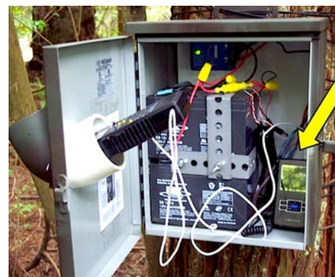
Figure 11. Second generation prototype long-duration field recording unit. Arrow points to programmable recorder.
