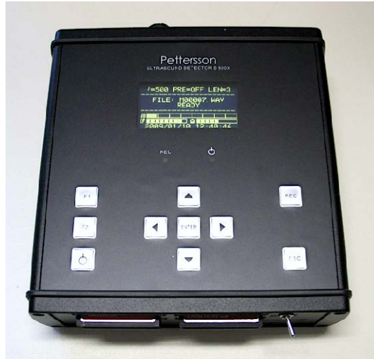
Figure 38. Pettersson D500X ultrasound recording unit intended for long-term, unattended recording of bat calls. The recorder is equipped with four slots for CF cards. The triggering system allows the device to start recording as a sound is detected. The recording length can be selected in steps from 0.3 up to 20 seconds. The recorder is normally operated in a low-power mode with no pre-trigger (i.e. the recording starts as the sound exceeds the chosen threshold level), but both pre-and post-trigger functions are available in the standard (not low-power) mode. This unit accepts an external microphone for flexible deployment.
