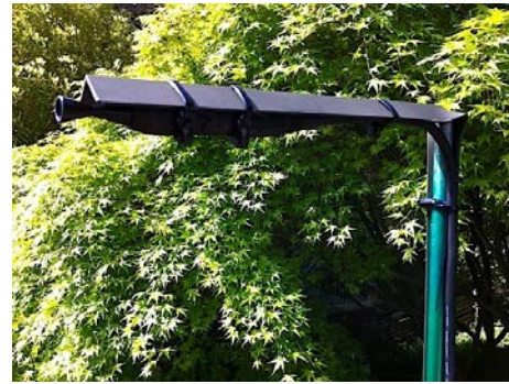
Figure 45. Bat detector remote microphones enable placement up and away from ground clutter and other surfaces that can generate echoes that distort recordings. Elevating the microphone can also increase the vertical coverage, from the microphone to the ground, and from the microphone upward; rather than just from the ground upward.
