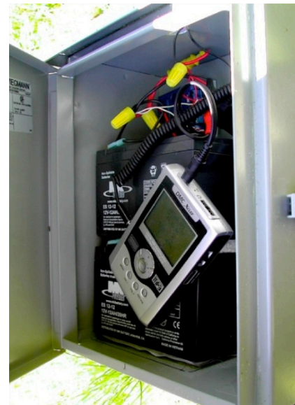
Figure 10. Initial mp3-based prototype long-duration field recording unit.
