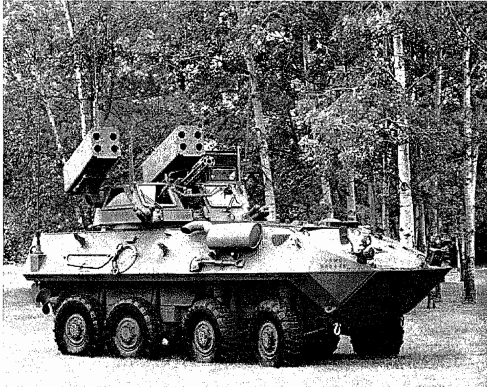
LAV-AD. Official USMC photograph. Armament: 25mm Gatling gun, 8 x Stinger Missiles.
