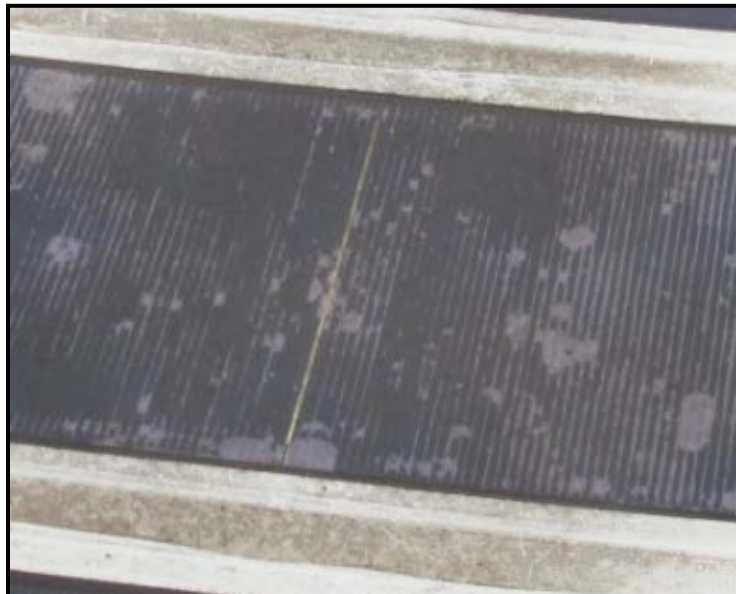
Figure-46: Evidence of PV delamination.
