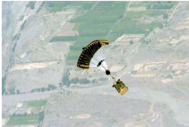
Figure 10. 2Klb capacity SCREAMER system deployed from a USAF C-130 in 1 st USAF/USA Combat JPADS airdrop in Afghanistan
