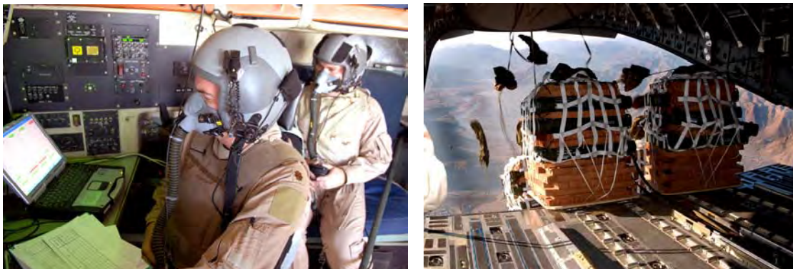
Figure 11. USAF Aircrew monitoring dropsondes data live on JPADS-MP Laptop (left) and multiple ICDS payloads deploying over Afghanistan (right)
