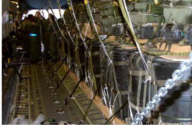
Figure 13. Picture of multiple CDS bundles rigged with WGRS in a C-17 aircraft
