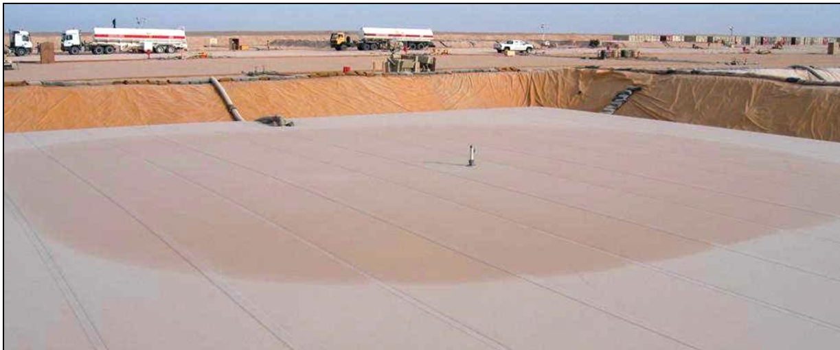
Figure 1. Deployed collapsible fuel storage tank showing fuel infiltration into nylon-woven fabric.
