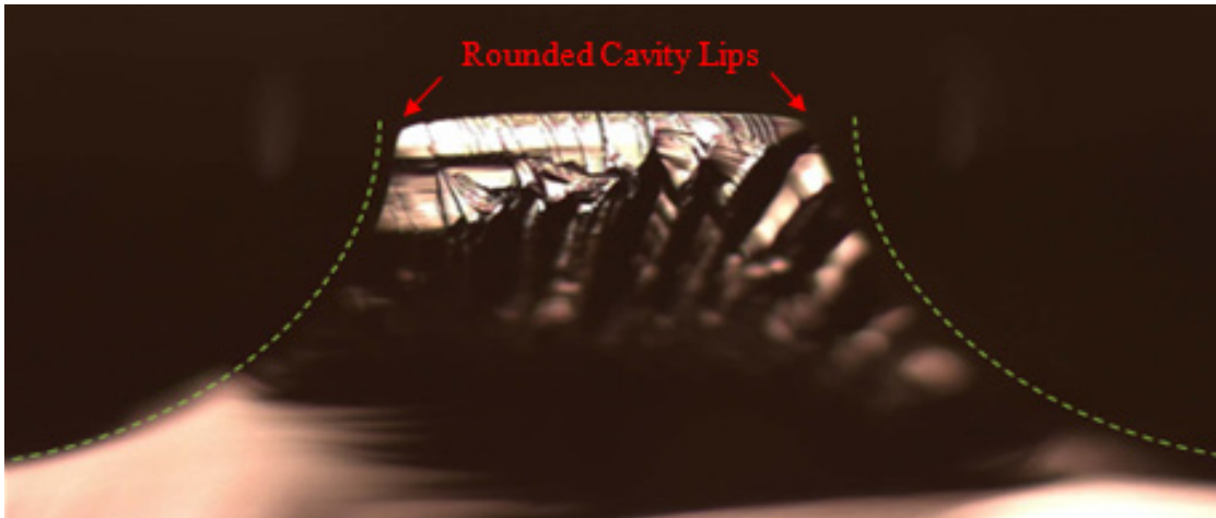
Figure 48. Cross-sectional profiles of two DSE-produced etch cavities after 10 minutes of 10:80:10 HNA polishing. The green lines represent ideal hemispherical profiles. The cavity lips near the center of the sample have achieved the desired rounded profile.
