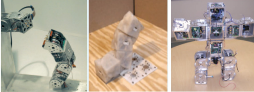
Figure 6. Left to right: PolyBot G3 from PARC, Molecubes from Cornell, and SuperBot from USC [12].
