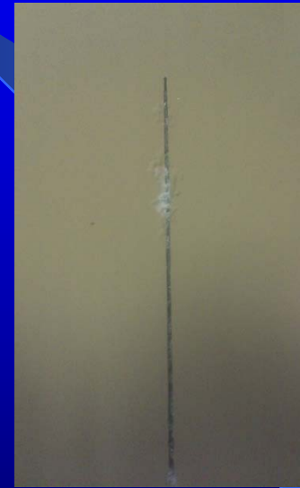
Anomag with e-coat and CARC after 5,376 hour salt spray test.
