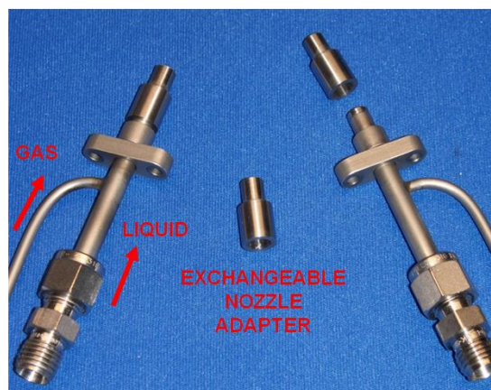
Figure 1. Photograph of axisymmetric aerated-liquid injector with exchangeable nozzle adaptors
