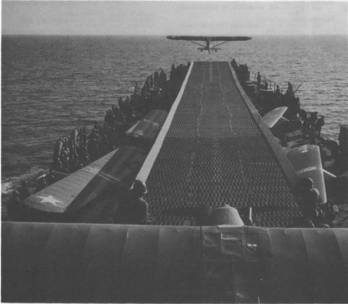
Figure 13. Army Piper L-4 Cub artillery observation plane takes off from an LST
