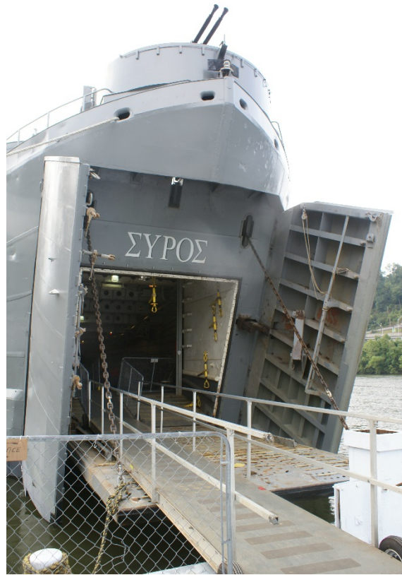
Figure 6. Bow Ramp and Bow Doors
