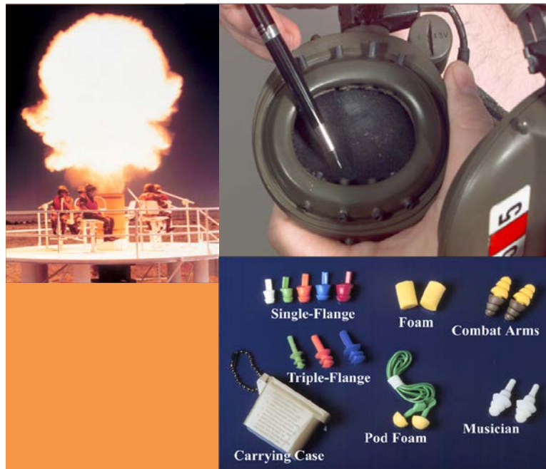
Figure 20. ABQ experiment showing five volunteers located 1.0 m from source in upper-left panel wearing an earmuff modified with eight tubes, shown in the upper-right panel. Other hearing protectors are shown in the lower panel, including the E.A.R. Foam and CAEs (green side is linear, yellow side is nonlinear).
