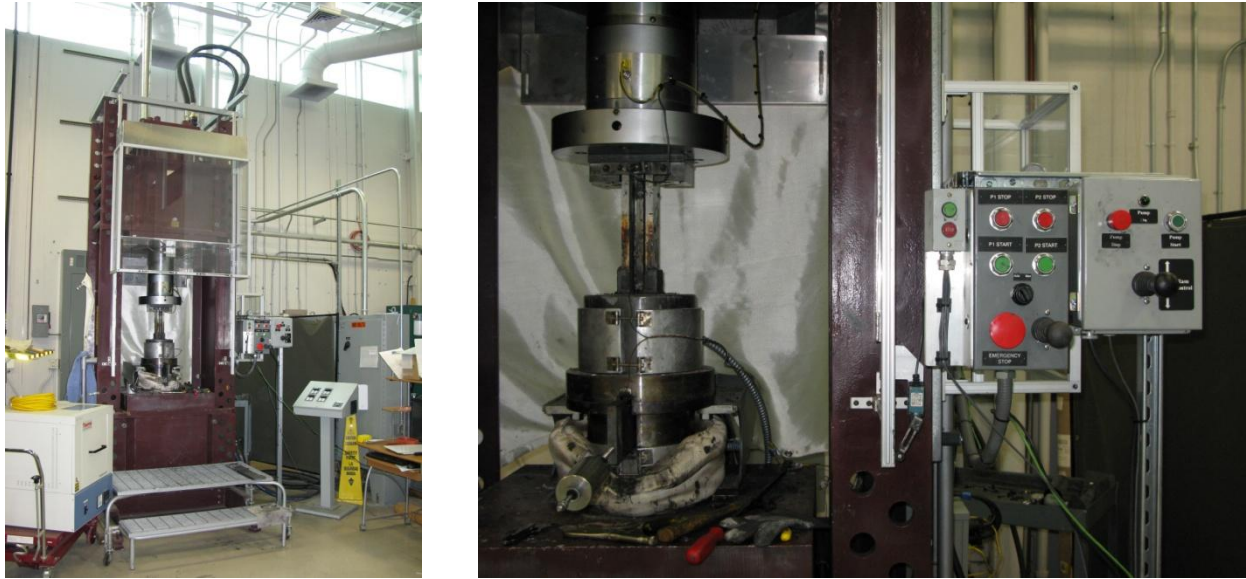
Figure 21. Photographs of the ECAE press facility located at ARL, Aberdeen Proving Ground, MD. Right photo shows the tooling die for 0.75- × 0.75- × 8-in billets and the control consoles.
