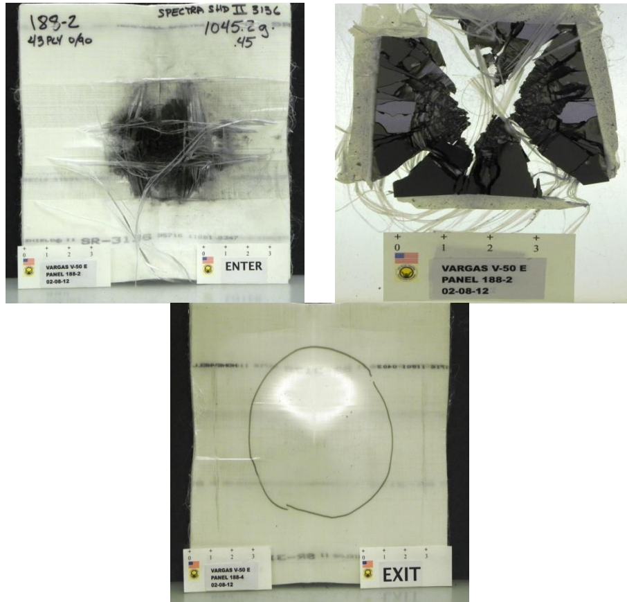
Figure 39. Baseline test panel; no Mg backing layer was used. Ballistic impact resulted in massive damage to tile, with the tile debonding from backing completely in most cases.
