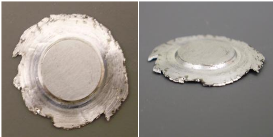
Figure 3. Picture of the HPT processing chamber as well as 10-mm-diameter ZK60 sample processed for six turns under 1-GPa pressure.
