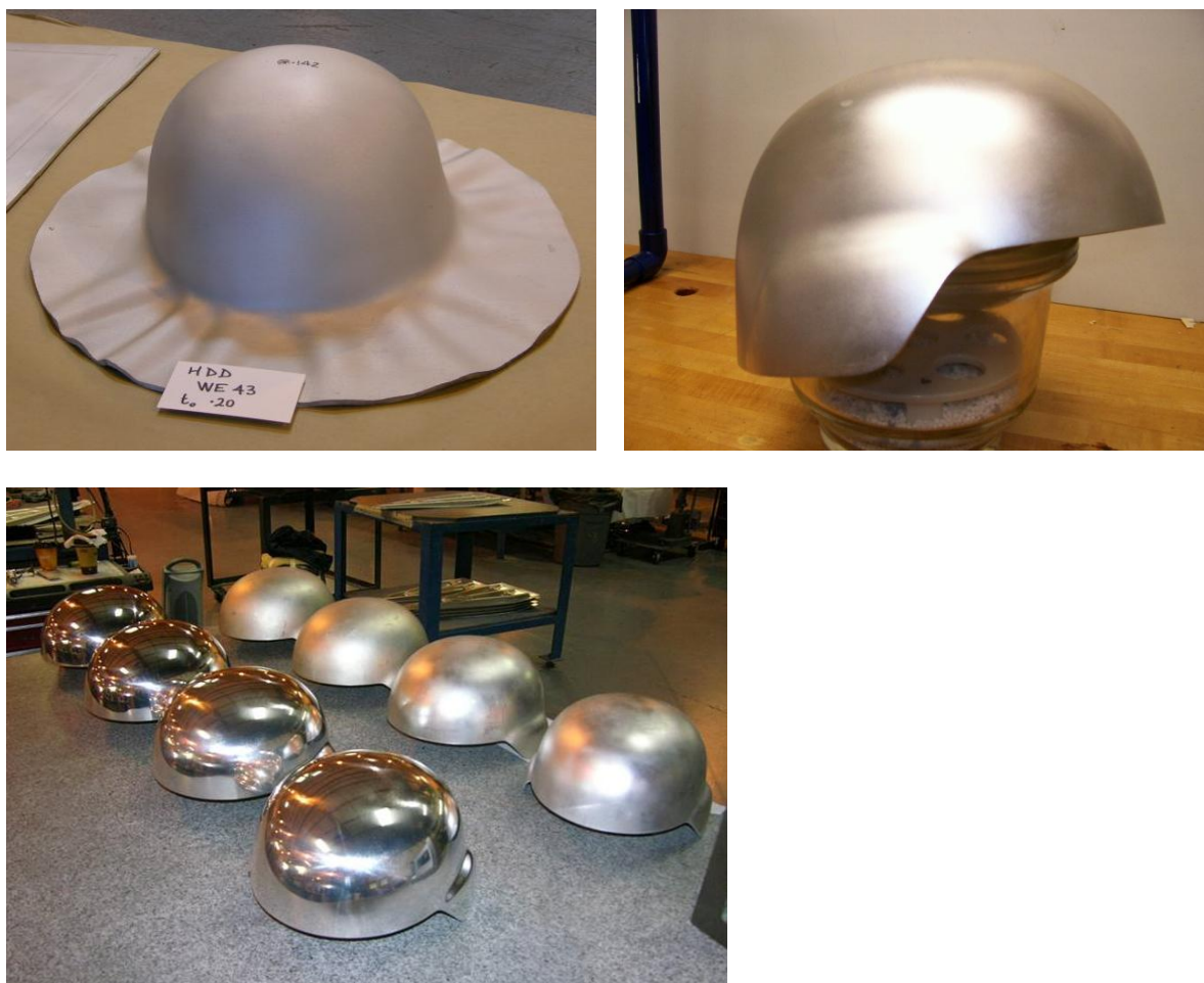
Figure 36. Representative helmet shapes made during series of superplastic forming trials, which resulted in a demonstrated ability to produce WE43 helmet shells with consistent quality.
