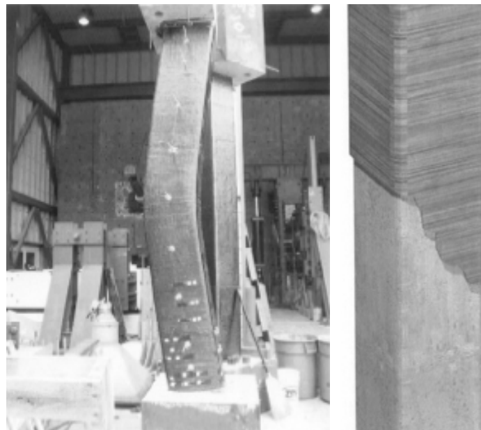
Figure 18. Column ductile performance enhanced by CFRP hoop wrap (left); wrapping detail (right) (Crawford, Malvar, and Morrill 2001).
