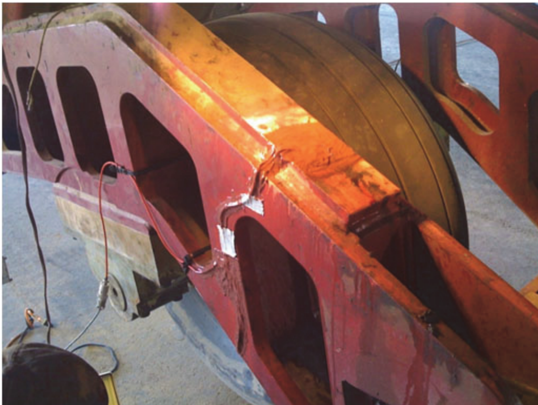
Figure 53. Carriage strain gauge arrangement.
