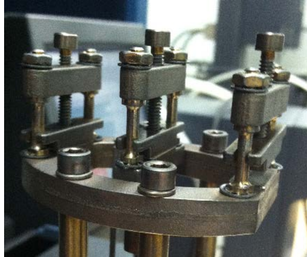
Figure 2. DCB test fixture including metal base.
