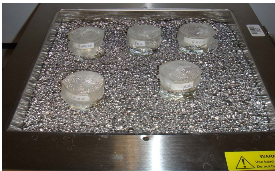
Figure 4: Lab Armor bead bath containing various flavonoids added to the model system and stored for 10 weeks at 50 °C.
