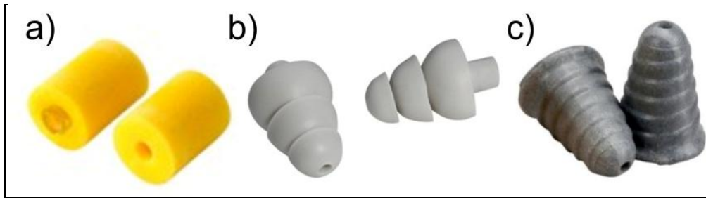
Figure 2. Earplug types used when measuring the impulsive noise attenuation provided by the ComTAC IV TCAPS headset. (a) 3M E·A·R Classic foam, (b) 3M UltraFIT triple flange, and (c) 3M Skull Screws.
