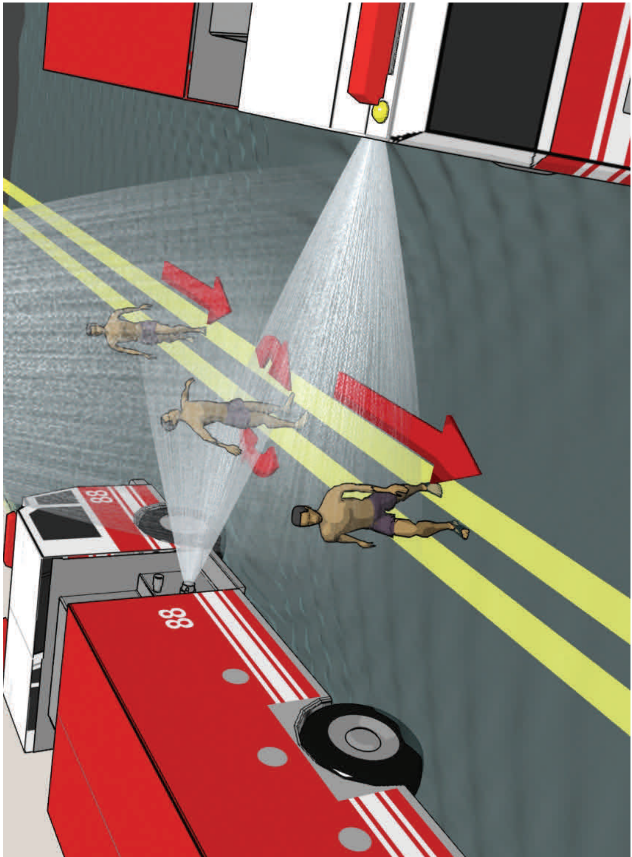
Figure F-7. Proper Decontamination Corridor Procedure
