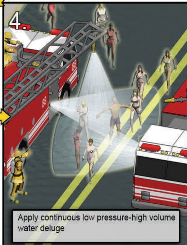
Figure F-2. Ladder Pipe Decontamination System (LDS)
