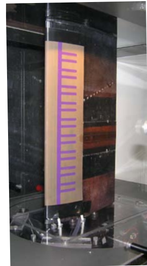
Figure 4. Plasma actuator configuration mounted in the wind tunnel.
