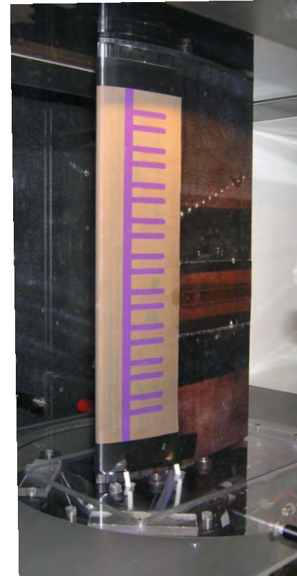
Figure 5.5. Plasma actuator configuration mounted in the wind tunnel.
