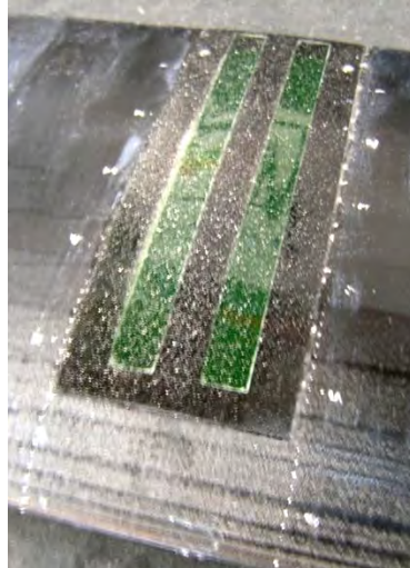
Figure 2.18 Example of S3F carrier filled and installed on Airfoil 2.
