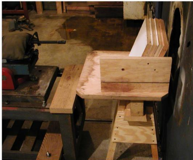
Figure 22. 5.56-mm deflection yaw-induction technique.
