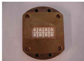
Figure 1: A double-sided SRR array inside a WR-90 waveguide section
