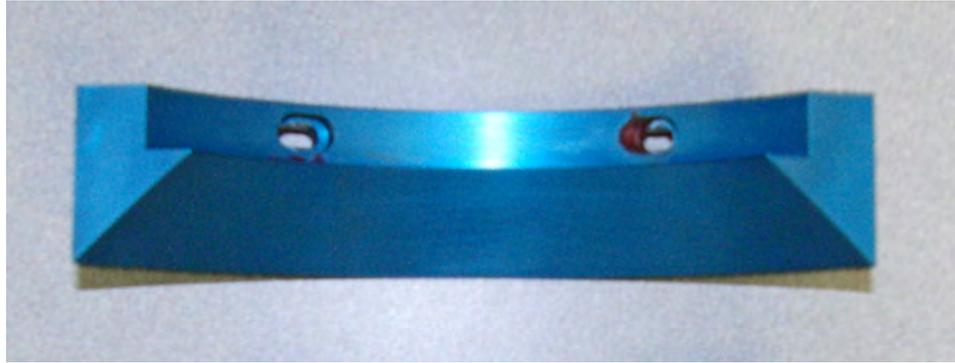
Figure 2.6: Wedge Cavitator used for Unswept Fin Testing
