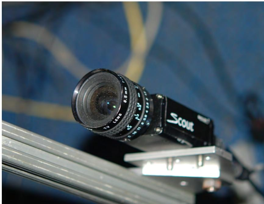
Figure C.4: Basler Scout color video camera used to observe the fin from the bottom of the tunnel, looking down the fin's span.
