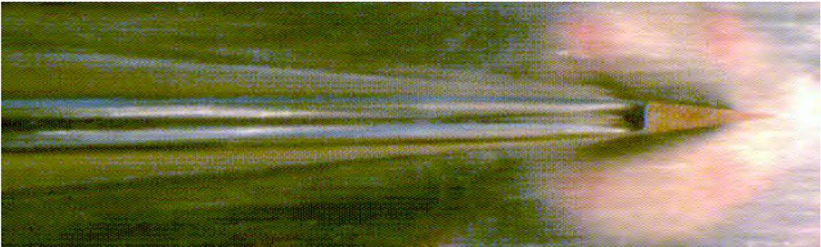
Figure 4.2: Base ventilated fin looking down the span from the fin tip,  $\alpha = 0^\circ$ , no sweep, 1 inch chord
