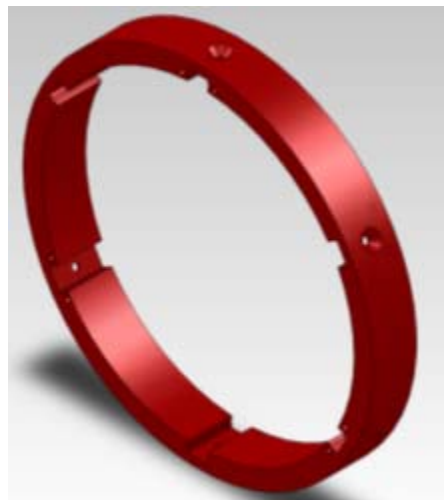
Figure 3.19: Combustor ring without top air inlets
