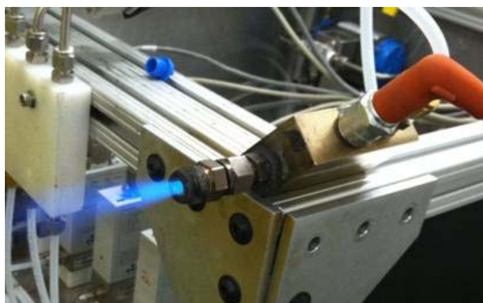
Figure 3.32: Ethylene torch with flame jet
