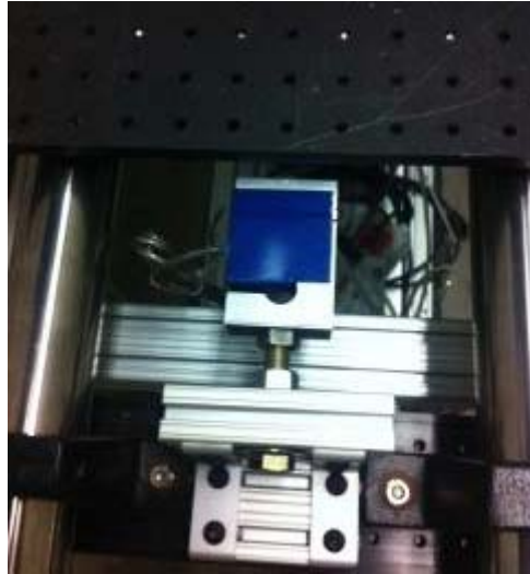
Figure 3.41: Load cell on the thrust stand
