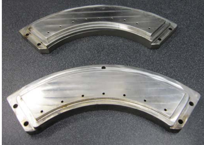
Figure 3.25: Instrumented inserts, inner face, front (top) and rear (bottom)
