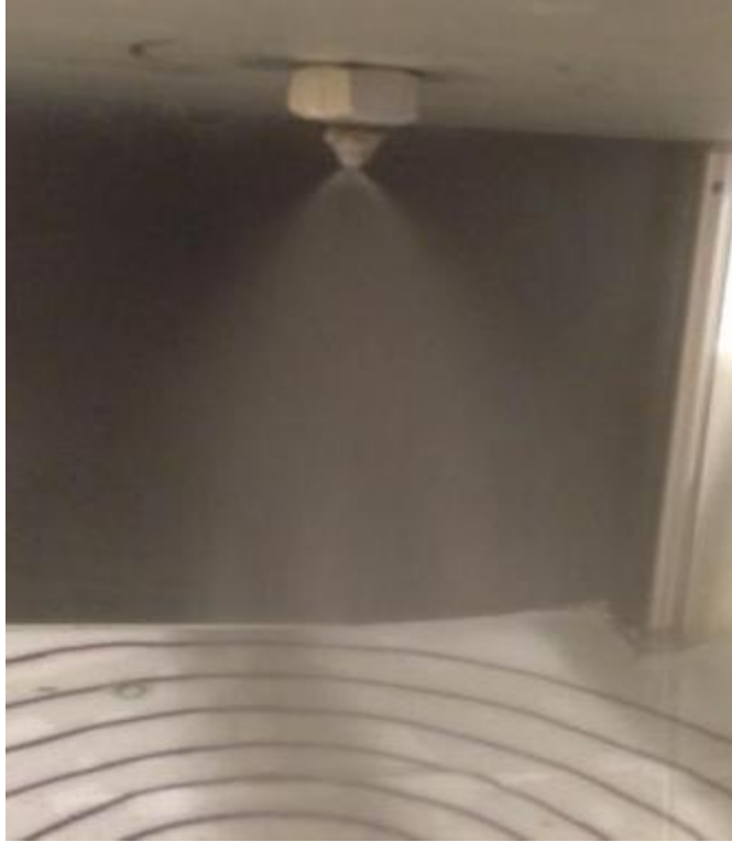
Figure 4.12: Fully developed fuel spray cone
