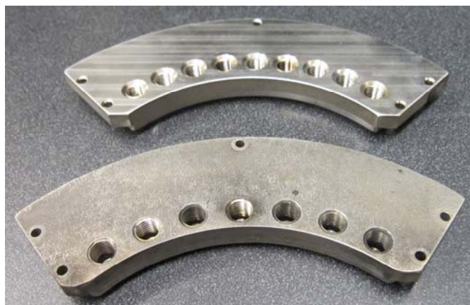
Figure 3.24: Instrumented inserts, outer face, front (top) and rear (bottom)
