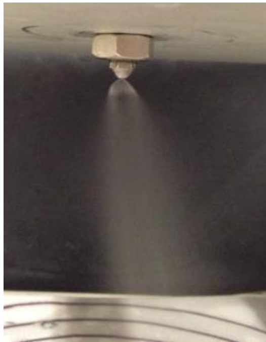
Figure 4.13: Partially developed fuel spray cone
