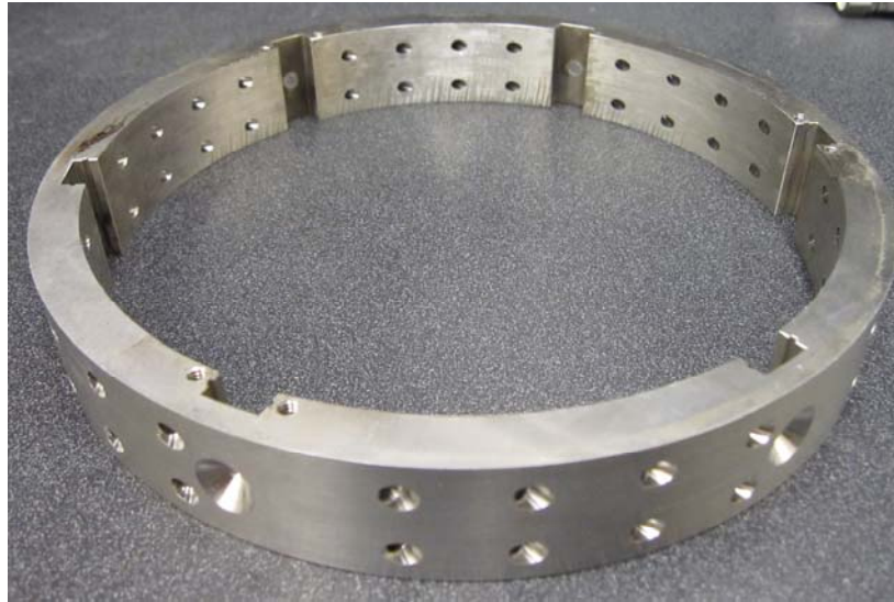
Figure 3.21: Combustor ring with top air inlets
