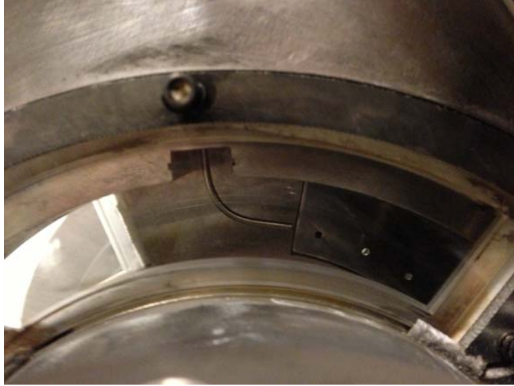
Figure 4.10: Pitot and static port locations
