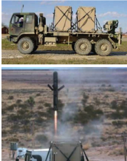
Figure E.11 NLOS-LS Container Launch Unit (C/LU) Shown Transported on a Truck and Subsequently Firing Its Precision Attack Munition (PAM)
