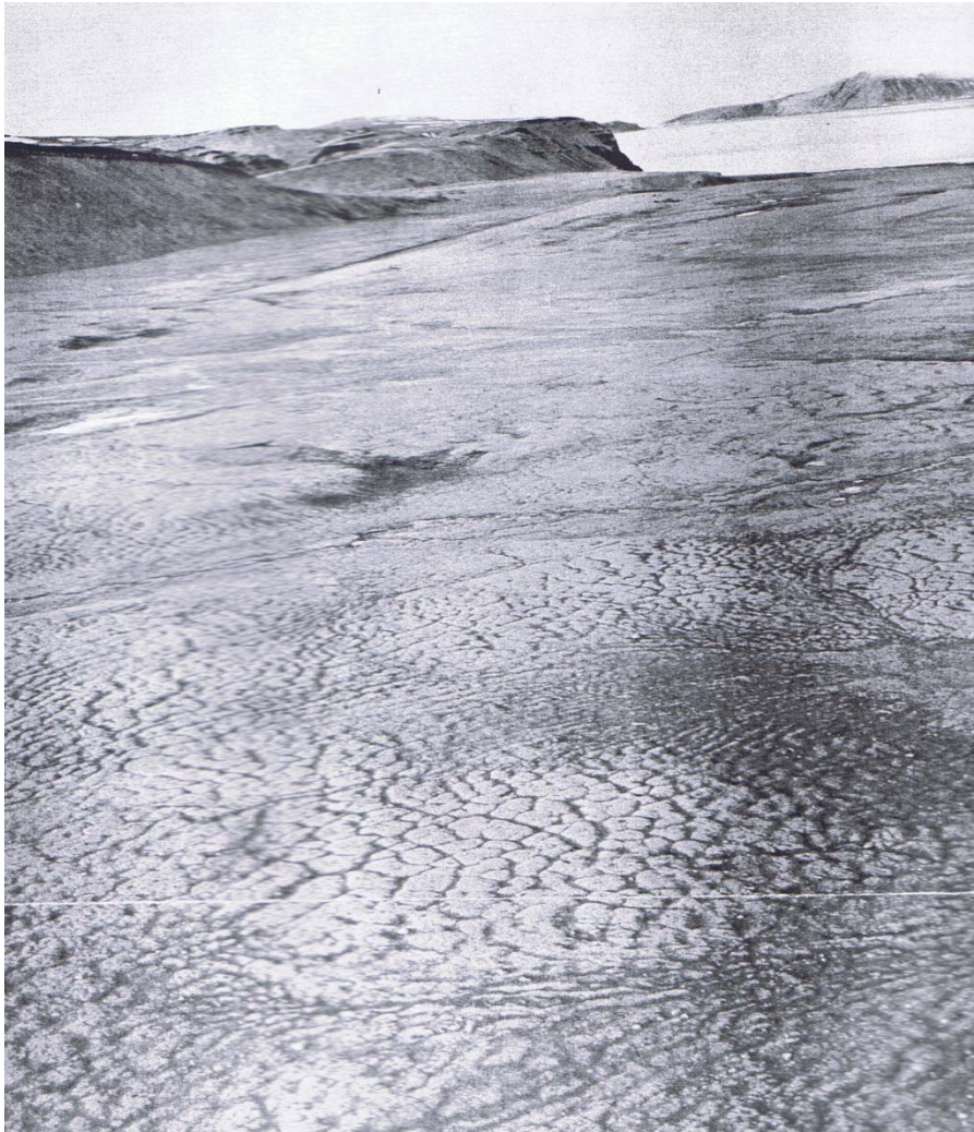
Figure 6. Aerial photo prior to Air Base construction looking southwest. The polygonal ice wedge networks are seen to extensively cover much of the valley.
