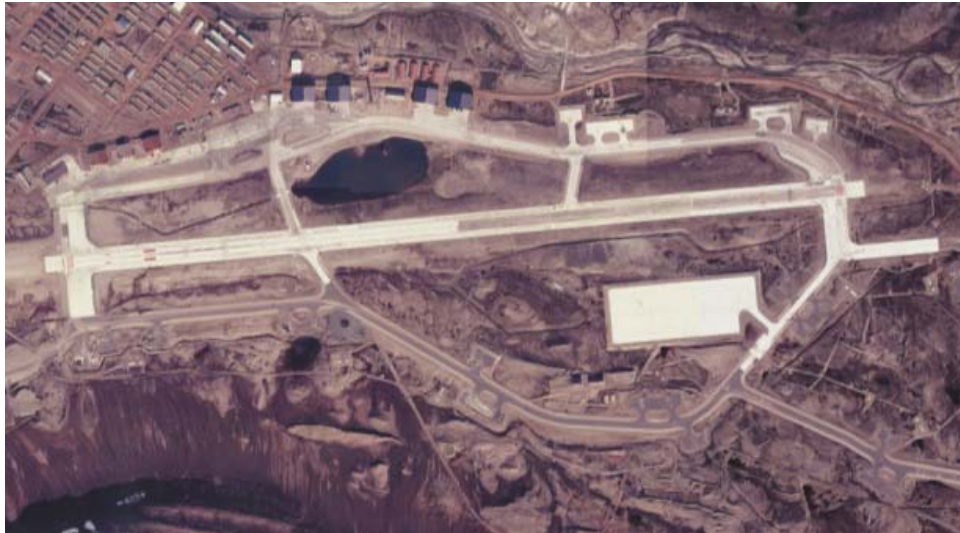
Figure 14. Undated photo of the airfield obtained from Thule personnel. The painting is in process during this photo. It is unknown if the dark pavement from approx. 50+00 to 100+00 is from wear or if milling or some other program is being conducted.
