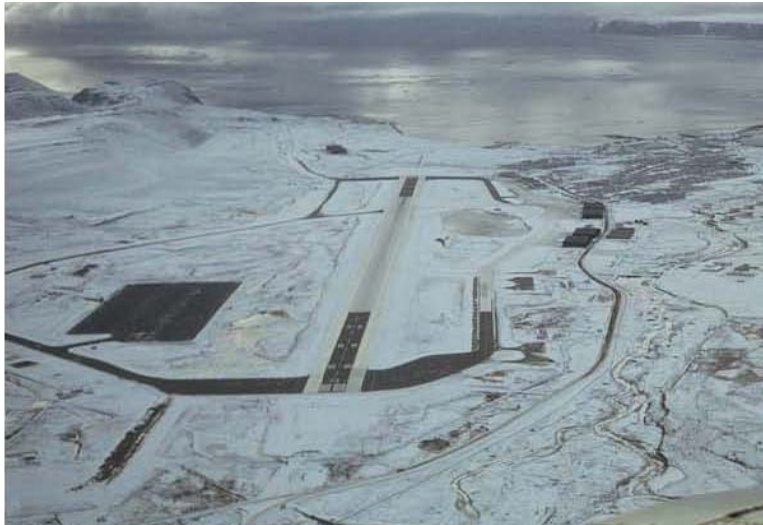
Figure 12. Airfield in September 1975 showing the extent of painting up to that time. The landing zones, 2000 ft from either end of the runway, are not painted nor is the 26 or 08 ends of Taxiway Alpha. This study found there was no information anecdotally, or in the literature, suggesting past thaw depression problems in these areas (Funder 1990).
