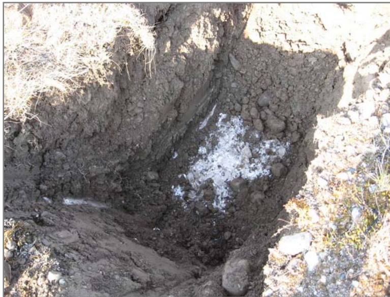
Figure 11. Test pit near Taxiway Bravo Extension. Wedge ice is seen at 5.5 ft depth.
