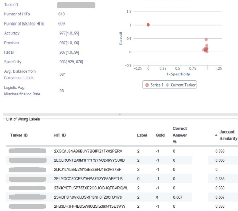
Fig. 4. A screenshot of an example individualized error report of a given worker’s performance (the worker’s ID is intentionally occluded in the screenshot). Such error reports are automatically generated for each worker and output as an interactive Google Web App Component that is hosted on our webserver. The top-left panel shows a set of numerical metrics characterizing the worker’s performance. The top-right panel shows a ROC plot (recall vs. 1-specificity) visualization. The bottom panel provides a listing of the worker’s specific mistakes (based on pseudo-gold aggregate labels). This listing promotes transparent performance assessment and allows workers to report any errors they find. Requesters can easily browse performance across individual workers as well as aggregate statistics. Workers are notified of the URL to their individual error reports via the Mechanical Turk API, though to avoid subsequent cheating on disclosed gold, only trusted workers are notified. Additional security measures are needed to ensure each worker’s error report is only accessible to the given worker.
