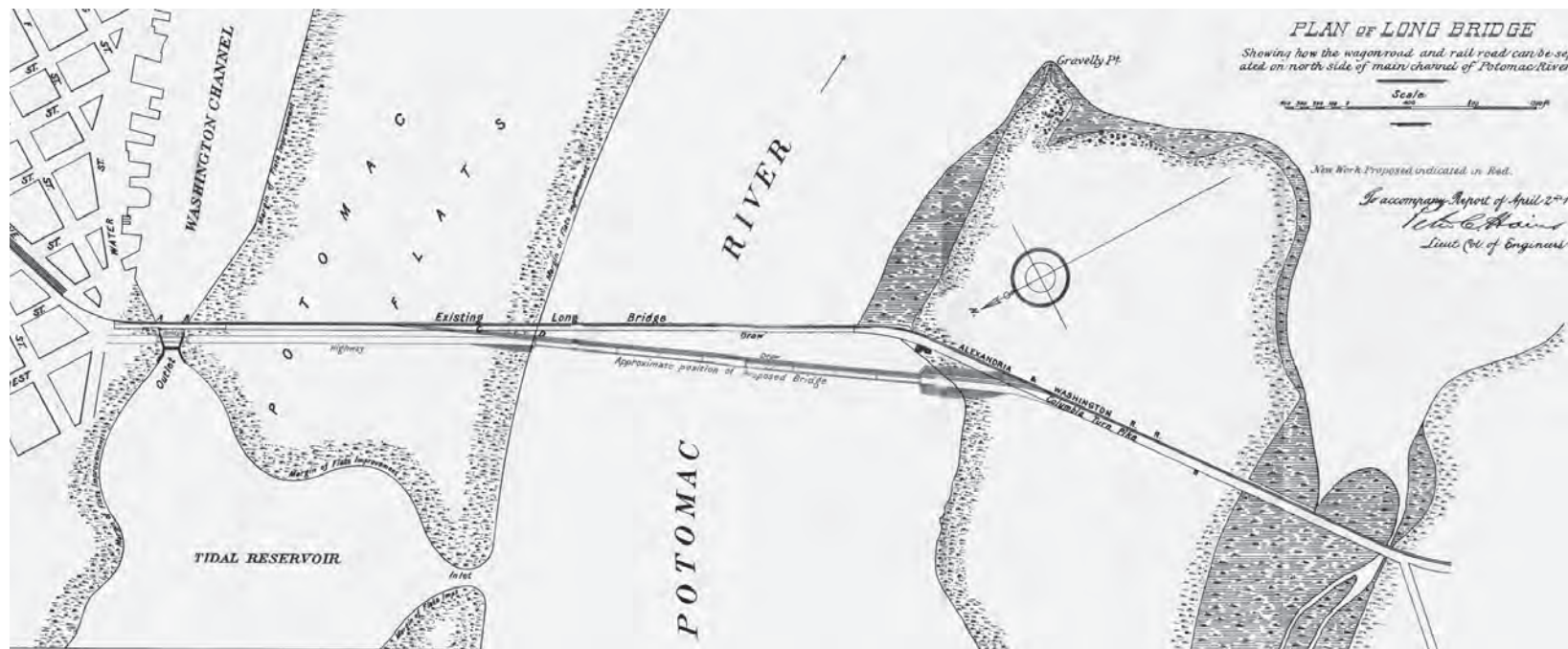
Plan of Long Bridge, showing the existing span and a modification proposed in 1890
