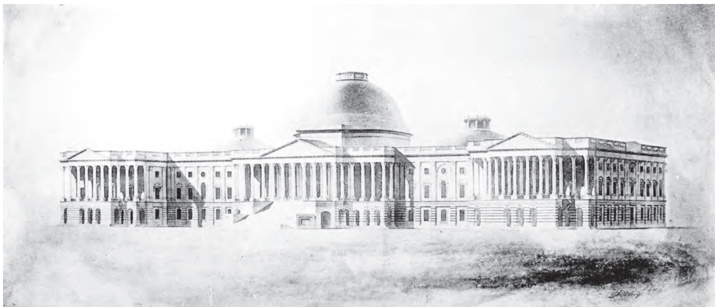
Corps of Topographical Engineers’ 1845 drawing of the extension of the Capitol, with porticoed lateral wings attached directly to the original building Architect of the Capitol, 63447
