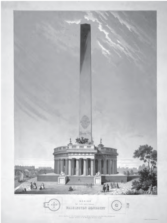
Although Robert Mills's 1845 design for the Washington Monument, lithographed by his son-in-law Charles Fenderich, called for a pantheon base 100 feet high and 250 feet in diameter, he designed the obelisk's foundations to carry the monument's weight without buttressing.
