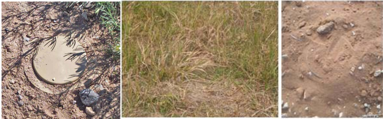
Figure 1: MicroObserver ® seismic sensors emplaced in ground
