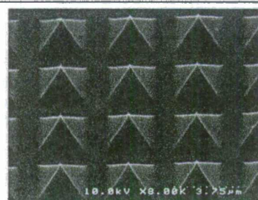
Figure 2.5: 2- \mu\text{m} pyramids produced with a 2- \mu\text{m} single oxidation
