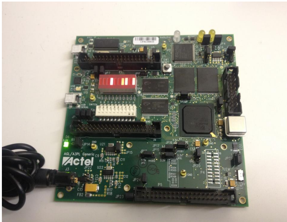
Figure 54. Actel ProASIC3 development board showing sequencer LED testing with TMR logic implemented.
