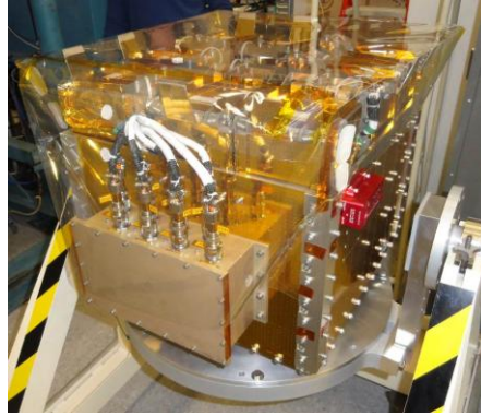
Figure 1. Final payload configuration and integration of NPSCuL with eight P-PODs.
