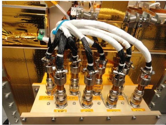
Figure 2. NPSCuL with associated Splitter Auxiliary Device (SAD) and external wiring visible.
