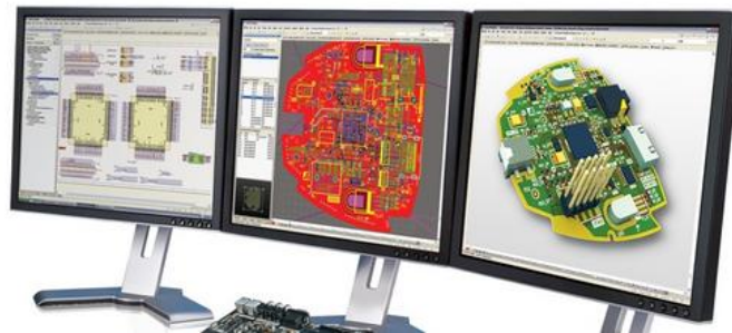
Figure 17. Altium Designer interface with separate schematic, 2-D PCB layout, and 3-D component placement views visible on separate monitors (From [73]).
