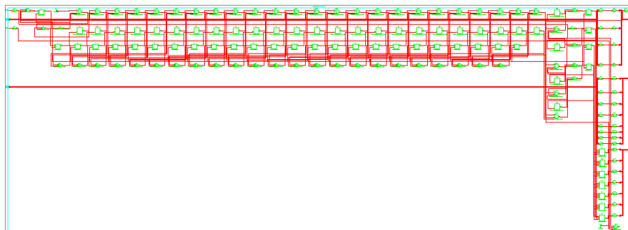
Figure 25. Default gate layout for baseline seven-segment LED counter.
