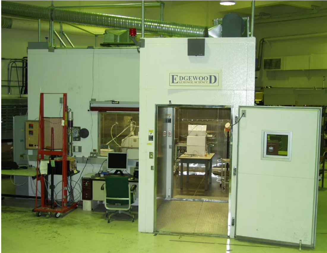
Figure 1 – Aerosol Deposition Chamber in Building E5951
