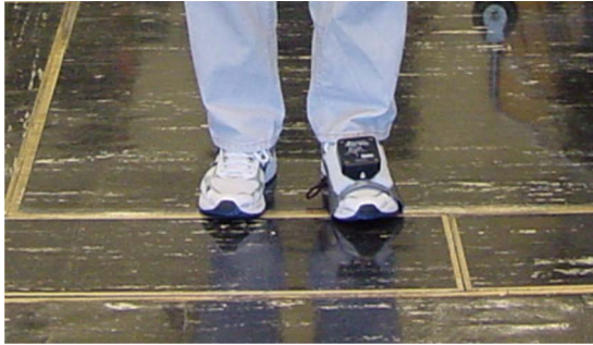
Fig. 1. Depiction of an inertial/magnetic sensor module attached to a foot for tracking foot motion during normal walking.
