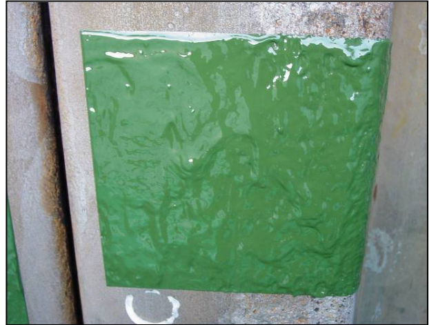
Figure 14. Typical test patch – PolySpec coating on San Diego steel sheet pile.
