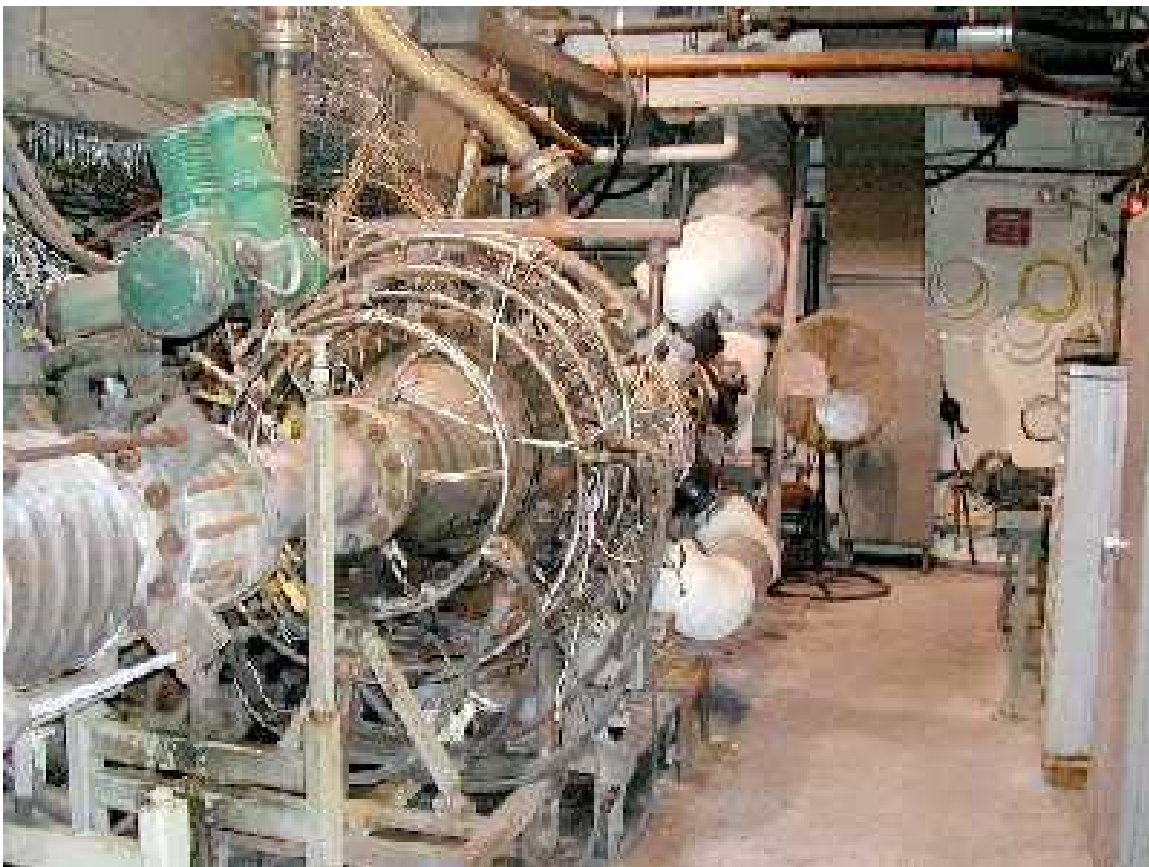
Figure 45. AE3007 Full Annular Combustor Rig 47
