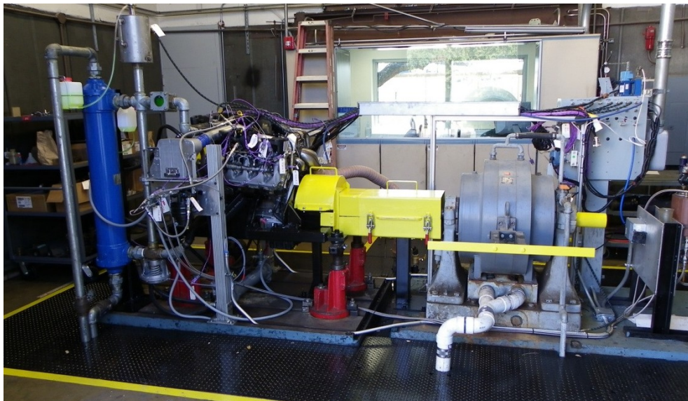
Figure 47. Ford 6.7 L Diesel Engine Test Installation
