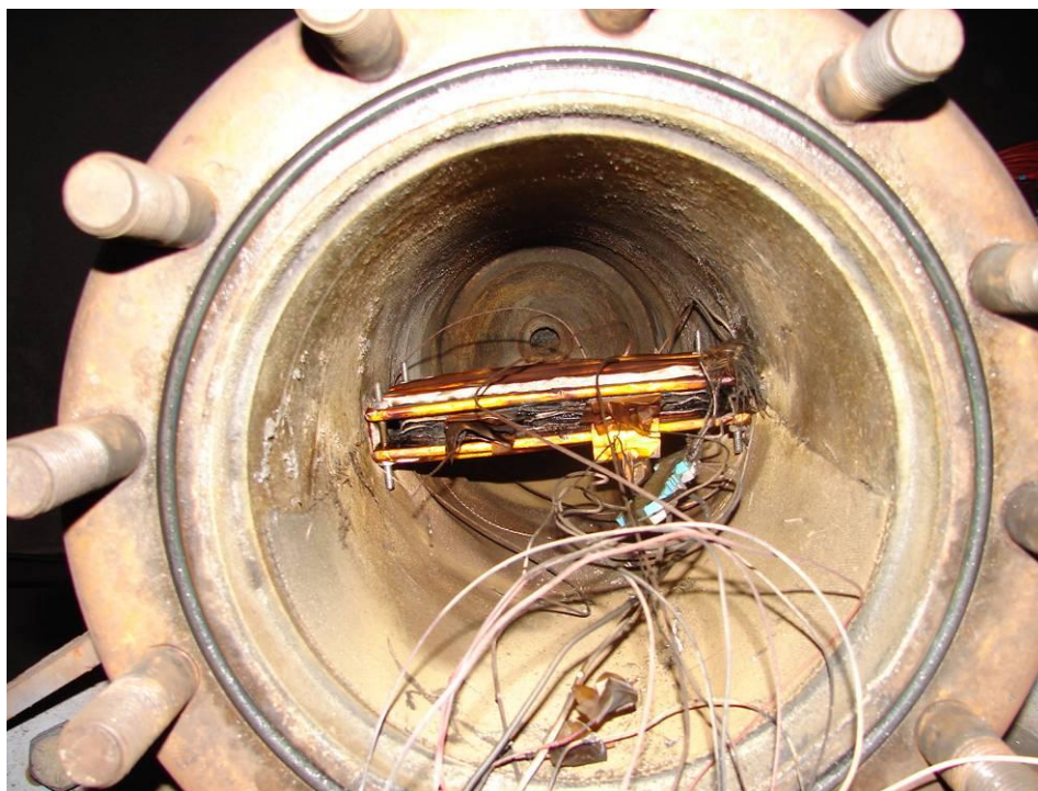
Figure 15: Altairnano Li-Ion Nano-Titanate Heat Tape Test Setup in the Test Bullet
