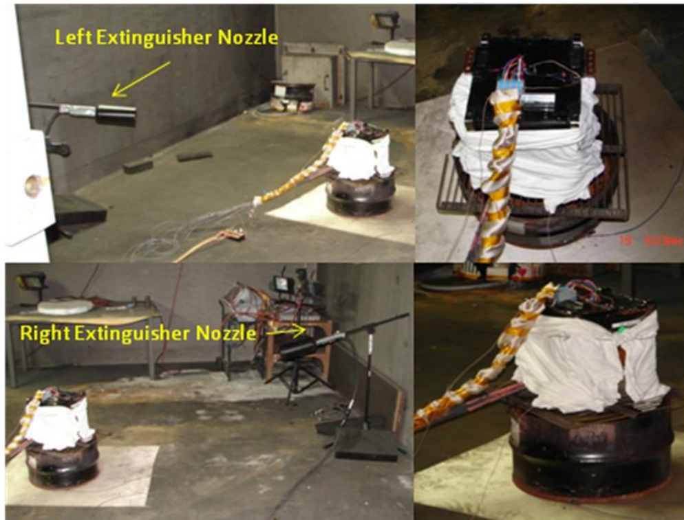
Figure 31: Mark I Module-Carbon Dioxide Extinguishing Test Setup
