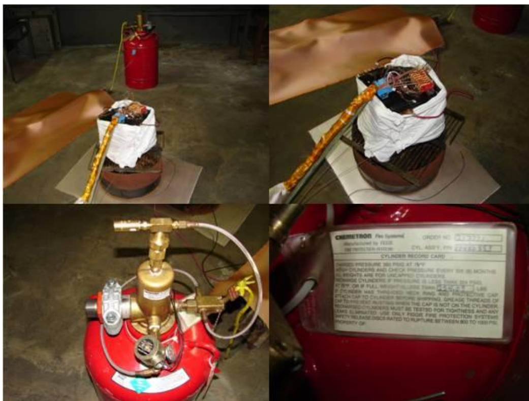
Figure 38: Mark I Module FM200 Test Setup
