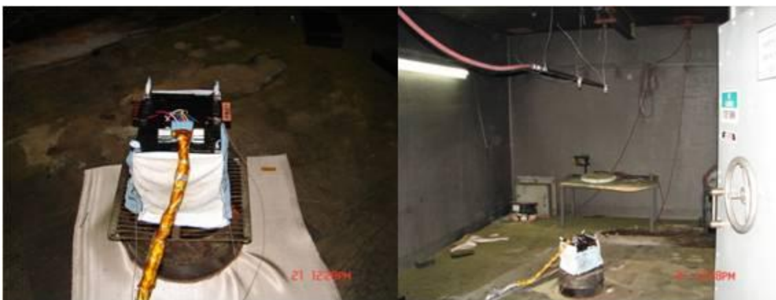
Figure 35: Mark I Module- Water Extinguishing Test Setup
