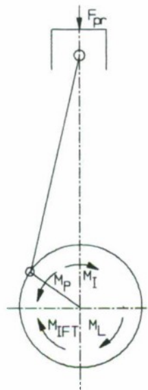
Figure 17. Balanced torques acting on the crankshaft
