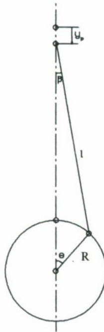
Figure 59. Piston reciprocating mechanism
