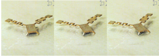
Figure 4. Still shots taken 3 s apart of robot turning counter-clockwise and translating at 1090 Hz.
