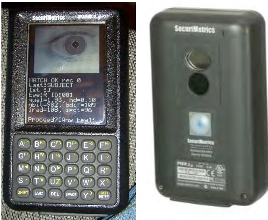
Figure 1: The L-1 Identity Solutions/SecuriMetrics PIER 2.3. This handheld device weighs 16 oz. and stores up to 400,000 templates in onboard memory for local matching. The back side of the PIER (right) shows the camera and the infrared illuminator.
