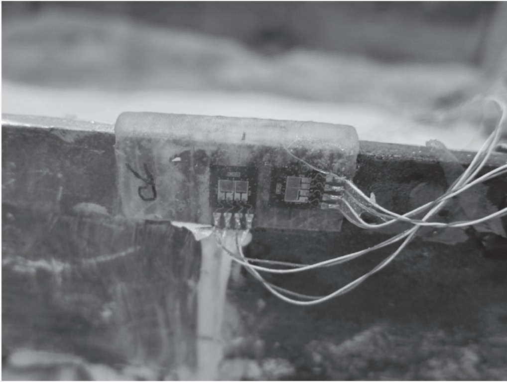
Figure 41. Instrumented polymer clip placed over two I-wall sections.
