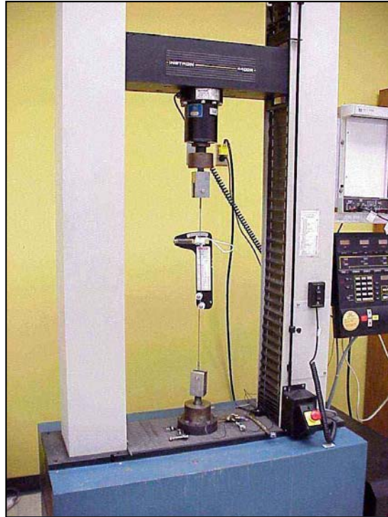
Figure 8-8: Test set-up used to correlate Loos Gauge vs. 1x19 and Dyform wire.
