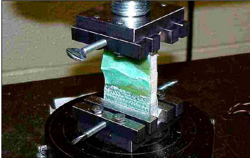
Figure 6-9: Compressive grips with failed specimen
