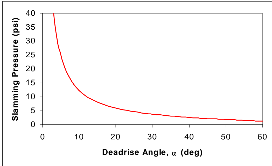
Figure 4-1: Maximum Pressure Due to Slamming ( u=10 fps)
