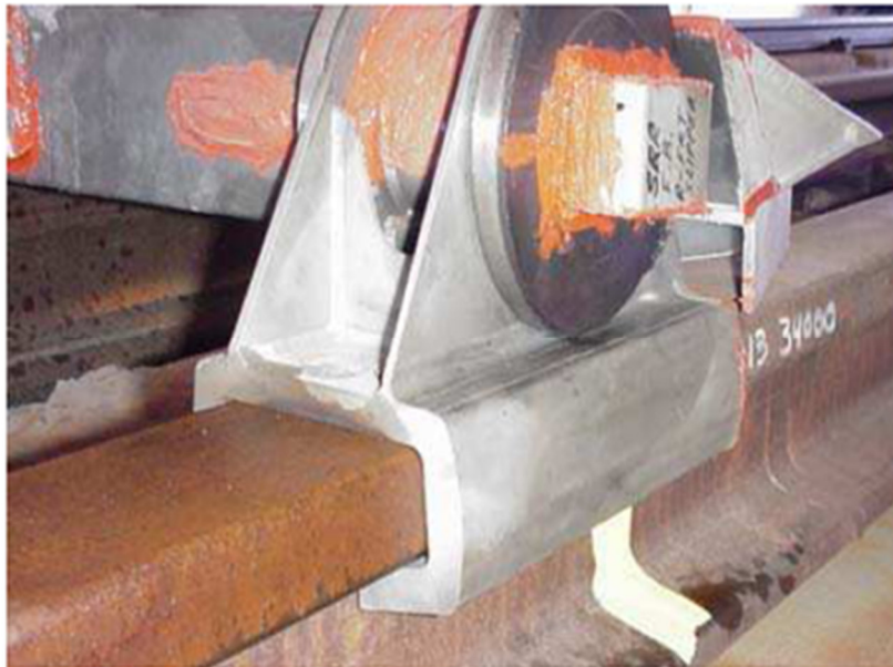
Figure 3: VascoMax300 Slipper attached to the 1080 steel Rail [3]
