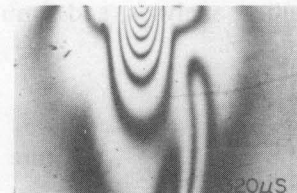
Optical Visualization of Impact-Generated Rayleigh Wave
