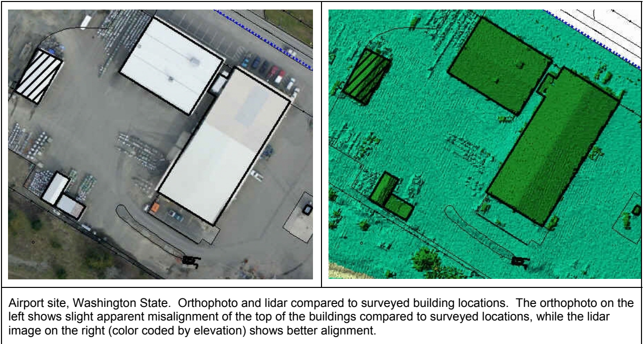
Figure 27: Apparent Misalignment of Tops of Buildings in Orthophotos
